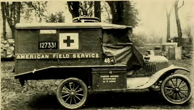
Side view showing sheet-iron apron and canvas storm-curtains to protect driver, top-rack for spare tires, side-box for tools and gasoline reserves, also front panel which swings open, allowing driver to arrange pillows for, or give water to, wounded on stretchers.
